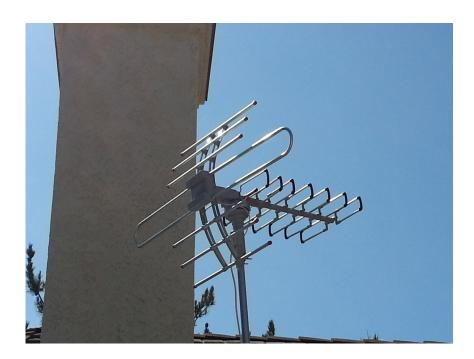
While searching the web I came across some cheap yagis HDTV antenna, which claim to operate from 45 to 860MHZ, have a 150 miles range (22-38dB gain) and come with a rotator. All this for for \$32.99 including shipping. I wanted to see how well would these antennas work on the 2m/70cm band, and see if I could modify them to work better on these bands. The particular model I got is the ESky HG-981 from amazon.
