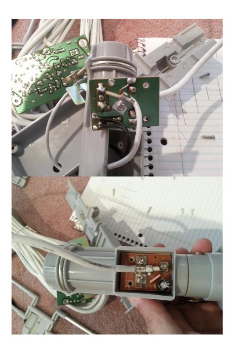
There is only a single coaxial cable leading into the antenna, which contains a filter to pass 12V
