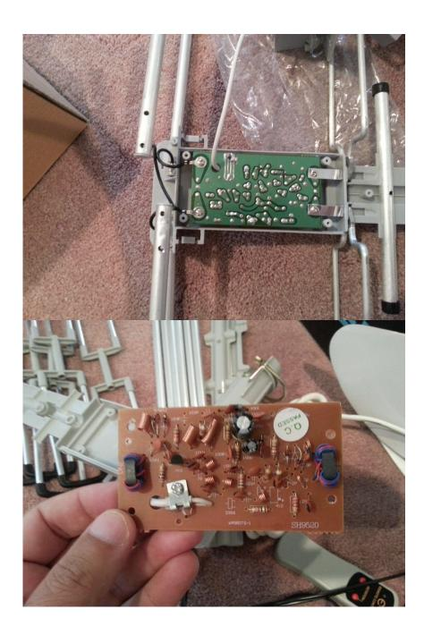
Before going into the radiating elements, the signal goes though another filter (a diplexer) which seems to split VHF and UHF signals into separate radiating elements from the signal feed line.
