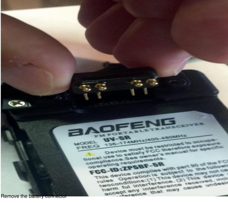
Remove the battery connector
